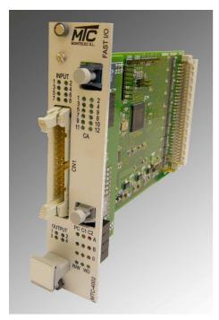
MTC-4002 is a fast counters and interrupts handler card designed to be used in simple applications as well as complex real-time controls.
