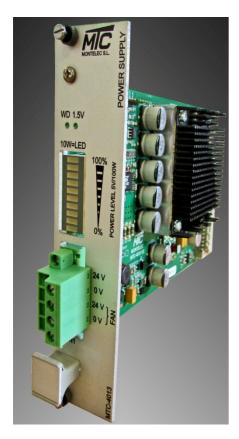
**MTC-4013** is a 24VDC / 5VDC and **100W** regulated power supply. Provides a reliable and continuous power supply.
