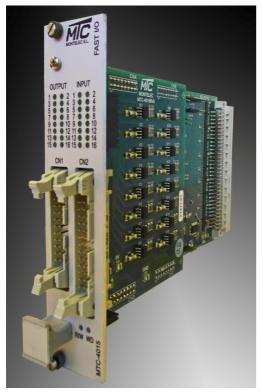
The MTC-4015 card is a configurable fast counters and interrupts card, as well as general purpose inputs and outputs. These counters can be used in both simple applications and complex real-time controls.
