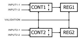
The validation signal can be done by a external signal or through a comparison of one of the counters.
