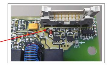
The connections are duplicated, alternated with a GND signal to increase immunity to electromagnetic noise.
